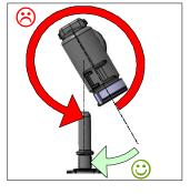
The line has to be positioned free of tension in the vehicle.
