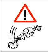
Protect quick connectors against dirt during assembly/ disassembly!
